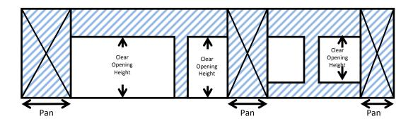
Refer to 2012 IRC Table R602.10.5 for minimum lengths of structural fiberboard braced wall panels for continuous sheathing.
